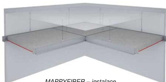
MAPPYFIBER – instalace na strop
